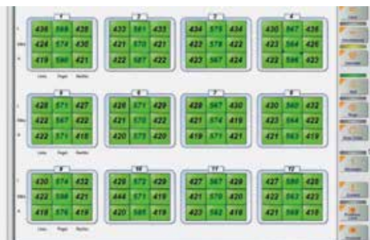
Blank Cooling Control temperature overview screen
