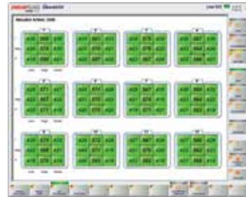
Plunger inner/middle/outer temperatures are kept automatically at set point (example shown: AIS 12 section TG)
