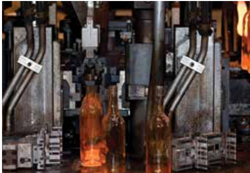
NIS final blow with FPS valve
