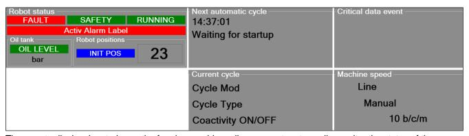
The remote display, located near the forming machine, allows operators to easily monitor the status of the FlexRobot when working around the forming machine.
